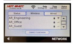
On the network screen, press "Wireless" and a list of available networks should appear. Select the appropriate network and press "CONNECT TO NETWORK"
