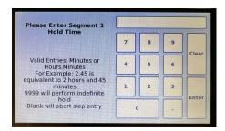
Enter segment hold time (Soak) in minutes or hours. Input examples below: 5 = 5 min, 5.0 = 5 hrs, 5.45 = 5 hrs and 45 min, 90 = 1.5 hrs
