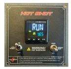
Press the "P" button one time to get to the "RUN" screen. Make sure it is set to "YES."
