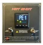
Press the "P" button one time until "PE1" appears. If an alarm is desired in this segment, set to "1."
