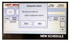
Adding a setpoint alert will sound an alarm when the setpoint temperature is reached.
