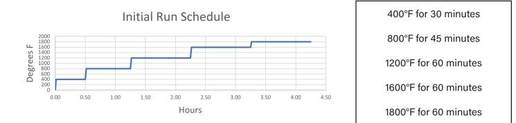
The run program will terminate and "COMPLETE" will display on the run screen. Allow the oven to cool back to room temperature on its own. Do not open the door or unplug the oven during this first heating/cooling cycle. After break-in, the door can be opened while in process to load/unload parts.
