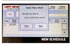
Adding a hold time alert will sound an alarm when the segment hold time has completed.
