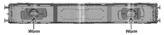
To expose drive worms and chassis for routine maintenance, simply pull the complete bogie assembly away from the chassis. The bogies are a 'pull-out' & 'push-in' fitting method. When refitting, ensure that the gear on top of the bogie tower meshes with the worm.
