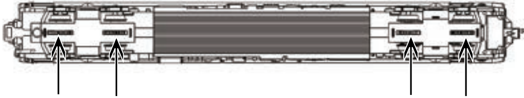
Normal oiling points into exposed gears without removing body
