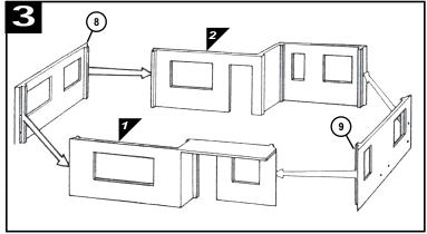
Cement side walls (8 & 9) to completed structures <1 & 2> to form the base of the building.
