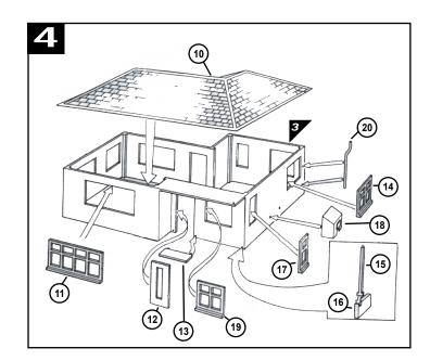
Cement roof section (10) into place and then cement windows (19 -17) into place as shown. Allow structure to dry. Then cement door (12), meter cover (18) and drain pipe (20) into place as shown. Leave to dry. Cement porch wall and roof support (15 & 16) together and then cement completed structure to edge of building and underside of roof as shown, using the locating pins and holes for exact position. Finally cement door step (13) into position, again using locating pins and holes.
