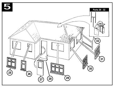
Repeat above procedure for rear of building using parts 25 - 31. Finally assemble the Chimney and Aerial (21 - 24) and cement to roof as shown.
