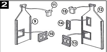
Cement windows (10, 13 & 14) into place on the side walls (9 & 12) remembering that the window sills face to the outside. Then cement chimney halves (11 & 15) into place as shown.
