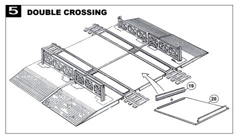
This kit will make a level crossing for a Single Track only. However, extra parts are included within the kit to allow you to make a Double Crossing (as shown) if two kits are used and joined together. Simply cement part (19) to extra base (20) and position
