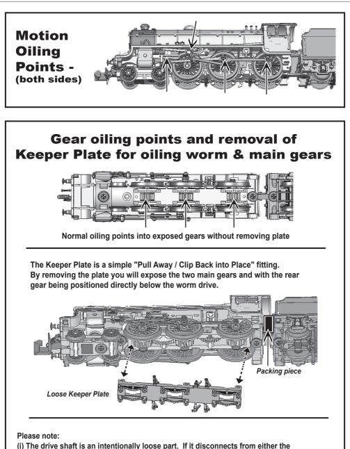
(i) The drive shaft is an intentionally loose part. If it disconnects from either the locomotive or tender it simply pushes back and clips into place using the slots in the enlarged cowling ends as the guides for the projections on either side of the drive shaft ends.
