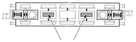
Add oil directly into the gears on the bottom side of the chassis
