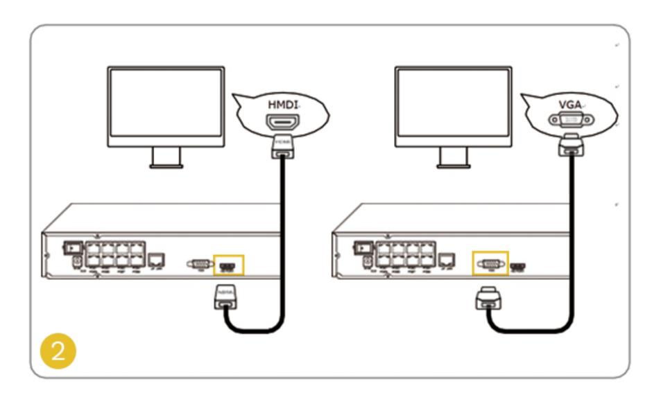
Connect the NVR to the monitor with a VGA or HDMI cable.
