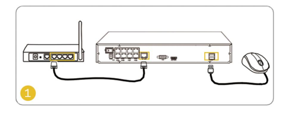
Connect the NVR (LAN port) to your router with an ethernet cable. Next, connect the mouse to the USB port of the NVR
