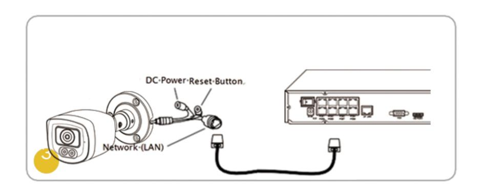
Connect the Camera to NVR with an ethernet cable.
