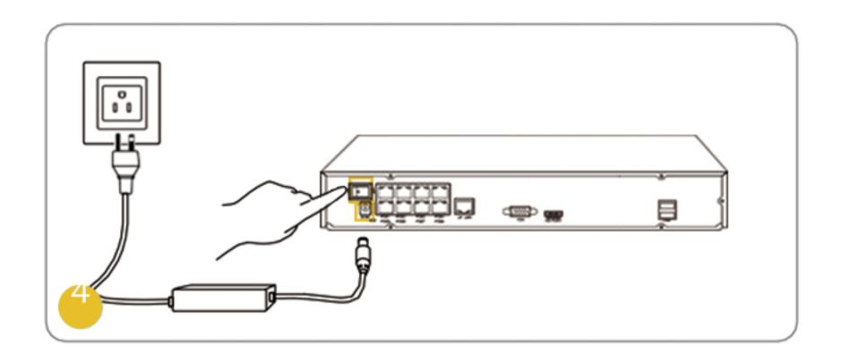
Connect the NVR to a power adapter and turn on power switch.
