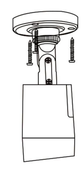
01/ Drill the screw holes in the ceiling according to the bracket.
