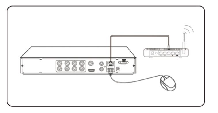
Connect the DVR (LAN port) to your router with an ethernet cable and connect the mouse to the USB port of the DVR
