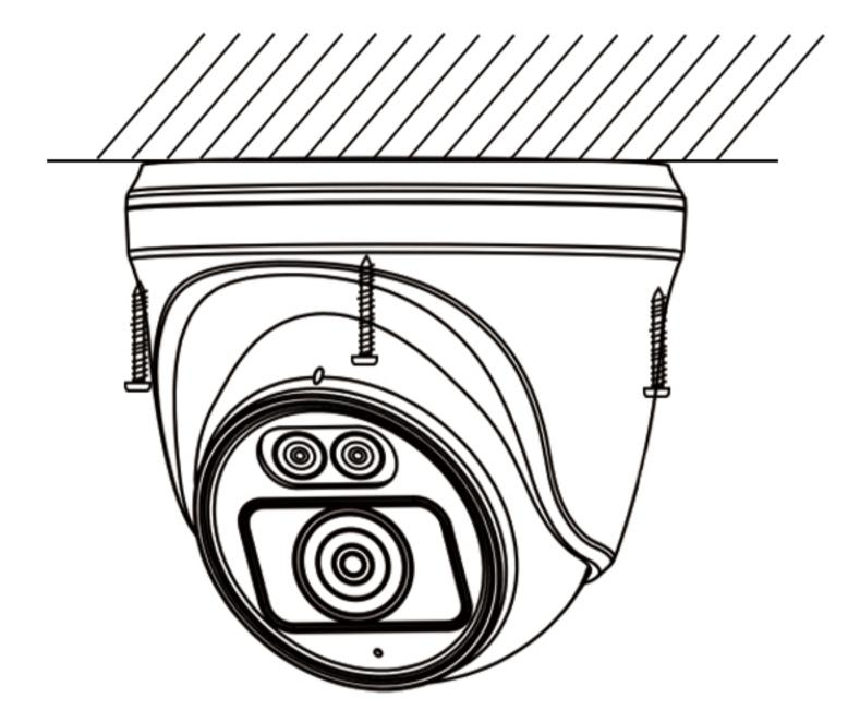
01/ Drill the screw holes in the ceiling according to the case.
