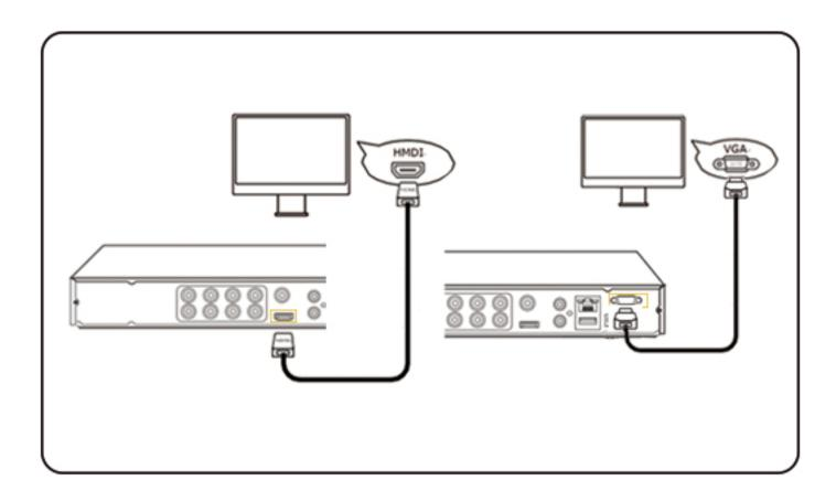
Connect the DVR to the monitor with a VGA or HDMI cable.
