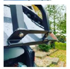
With rear door open, align bottom of the ladder parallel to the bottom of rear hatch door, Attach bottom bracket, with provided screws, to base of ladder (over the lip of the bottom door hatch), as shown in **Photo 3.**
