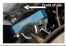
13. Reinstall the lower control arms to the subframe. This kit will get the rear alignment close to factory specifications but for proper handling characteristics and maximum tire life, we highly recommend an alignment after installation.
