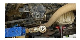
2. Remove the bolts for the subframe supports, these will be at the front of the rear subframe. On some models, there is an additional brace going to the chassis of the car, you will want to remove this as well
