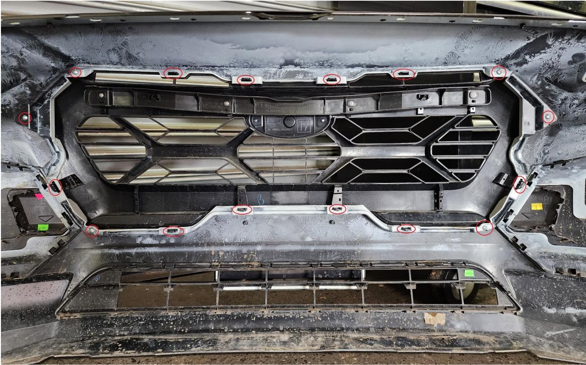
Test fit bumper, snug fairlead plate to the bumper, and tighten. Mark for trimming from back side of bumper though fairlead plate.
