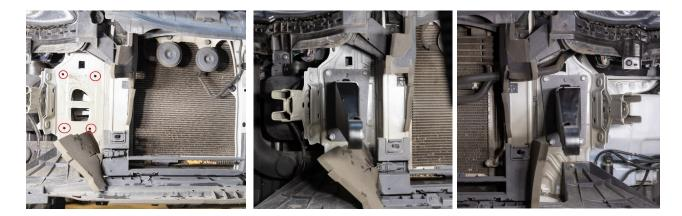
Install center plate and loosely install fairlead plate for test fitment. Install winch and wiring per manufacturer instructions.
