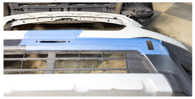
Test fit bumper, snug fairlead plate to the bumper, and tighten.
