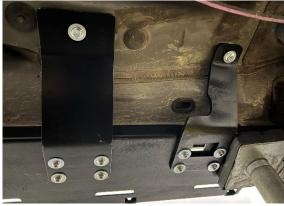
5. (OPTIONAL) NOTE: For a faster install you may let the bottom slider hang from the mounting bracket, attach the slider top to the base using supplied M6 button head bolts and serrated nuts (only a couple of threads on these bolts), support the slider to pinch weld, then use the slider as a template to drill the ¼" holes in pinch weld (a right angle drill is recommended, start with a smaller 1/8" bit then step up to ¼" or 9/32"). Then skip to step 8.
