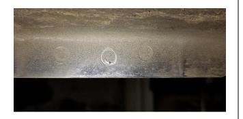
6. We recommend using a 1/8" drill bit to start drilling the mounting holes in the pinch weld and then stepping up to a 1/4" or 9/32" drill bit. Some paint is recommended on the newly drilled holes to prevent corrosion. Repeat the process for the other side.
