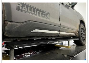
8. Rotate the rock slider assembly up in to place and use jack stands to support the rock sliders while you install the M6x40mm bolts through the pinch weld. Use a 10mm wrench to hold the nut through the cut out while you start the bolt from the inside of the pinch weld. Once all the bolts on one side are installed, tighten the bolts that go through the pinch weld.
