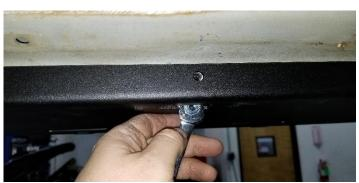
9. Once the bolts through the pinch weld are tight, tighten the outer M6 screws. The nuts are serrated so you do not need to hold them while you tighten the bolts.
