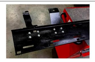
4. Take the rock slider base and brackets to their respective sides and start the bolts for the braces. The front brace will use the included M6x40mm bolts, 10mm spacers, and M6 fender washers. The center and rear braces will use the included M8x30mm bolts and M8 washers.
