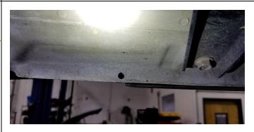
7. Loosely reinstall the rock slider base and let it hang from the bolts. Carefully install the rock slider top (they are the same left and right) and start the bolts to hold it to the base using the supplied M6 button head bolts and M6 serrated nuts.
