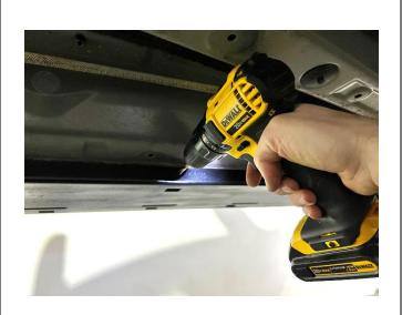
(STANDARD INSTALL) Rotate the rock slider base into position and mark the holes to be drilled in the pinch weld using a scribe or pick tool. It is helpful to support the front and rear of the rock slider base with jack stands while you mark the holes. Once you have marked the holes, remove the rock slider base and center punch near the bottom of the mark. Repeat the process for the other side.
