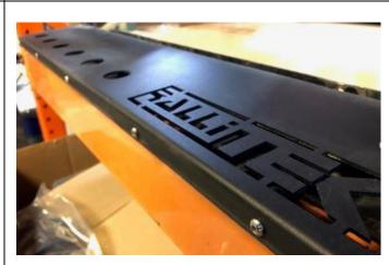
Install the plastic under trays. Remove the M6 bolt at the front bracket to hold the plastic in place, the plastic will go on the bottom of the bracket.
