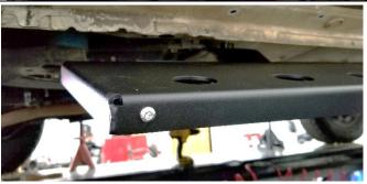
8. Rotate the rock slider assembly up in to place and use jack stands to support the rock sliders while you install the M6x40mm bolts through the pinch weld. Use a 10mm wrench to hold the nut through the cut out while you start the bolt from the inside of the pinch weld. Once all the bolts on one side are installed, tighten the bolts that go through the pinch weld.
