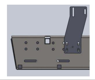
4. Take the rock slider base and brackets to their respective sides and start the bolts for the braces. The front brace will use the included M6x25mm bolts with 2 M6 fender washers and the rear will use the included M8x30MM bolts/M8 washers for the rear two mounting holes, and the longer M8X40MM bolts/M8 washers for the third mounting hole.
