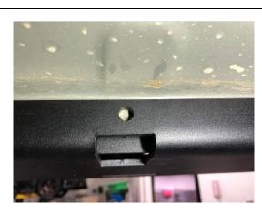
STANDARD INSTALL: Rotate the rock slider base into position and mark the holes to be drilled in the pinch weld using a scribe or pick tool. It is helpful to support the front and rear of the rock slider base with jack stands while you mark the holes. Once you have marked the holes, remove the rock slider base and center punch near the bottom of the mark. Repeat the process for the other side.
