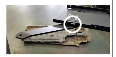
Install the braces onto the rock slider bases using the supplied M8 button head bolts and serrated nuts as shown. Be sure that the front brackets angle upwards from the base.
