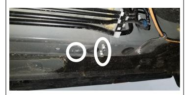
5. (optional) NOTE: For a faster install you may let the bottom slider hang from the mounting bracket, attach the slider top to the base using supplied M6 button head bolts and serrated nuts (only a couple of threads on these bolts), support the slider to pinch weld, then use the slider as a template to drill the 1/4" holes in pinch weld (a right angle drill is recommended). Then skip to step 8.
