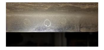
6. I recommend using a 1/8" drill bit to start drilling the mounting holes in the pinch weld and then stepping up to a 1/4" or 9/32" drill bit. Repeat the process for the other side.
