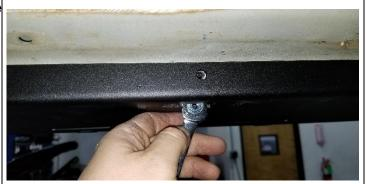
NOTE: the rock sliders may need to be manipulated up or down to get the bolts to start into the nuts. I recommend applying a little tape to keep the nut on the wrench during this process.
