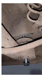
3. Remove the heat shield bracket and lower 1 hole. Use the supplied 10mm spacer and M6 bolt to reattach the bracket to the subframe.
