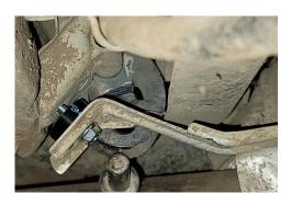
4. Remove the lower emergency brake cable brackets and reinstall using 10mm spacer and m8x1.25x30 bolt
