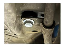
5. Going back to the 4 main subframe bolts, lower the jack down and remove 2 of the bolts. Slip the long spacer in between the subframe and the chassis and reinstall the bolts. Do the same to the other side but do not fully tighten the bolts at this time.
