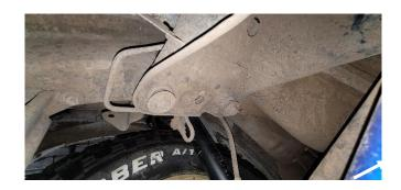
2. Using a 17mm and 12mm socket remove the front braces. Replace the 17mm bolts with the supplied 120mm bolts
