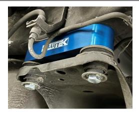
6. Moving to the front bolts, install the round spacers between the subframe and the chassis. Before installing the 120mm long bolt, install the new subframe brace brackets using the factory 12mm bolts. The one with the "L" will go on the driver side.
