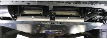
6. Optional step, you can cut the front of the factory splash guard to fill in the gap between the bumper and the skid plate. Tape a line approximately as shown, cut the front of the splash guard off and reattach using the clips you removed earlier.
