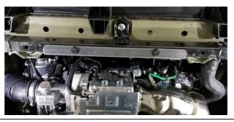
3. Using a pair of wire cutters, remove the turbo air duct off of the factory splash guard.
