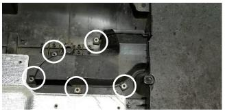
4. Using the supplied M6 hardware, attach the turbo air duct to the RalliTEK skid plate
