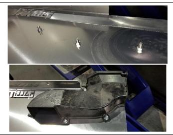
5. Using 2 of the supplied 60mm long M8 bolts, attach the front of the skid plate as shown, and then install the remaining 60mm long M8 bolts to the rear of the skid plate. Tighten all of the hardware once all 4 bolts are started.
