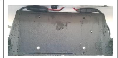
2. Install your license plate and RalliTEK license plate frame using the remaining 2 screws in the kit.
