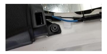
4. Remove the 4 nuts that hold the rear exterior trim piece to the hatch (2 are easy to see and the other 2 can be accessed through holes in the inner structure), unplug the wire harness and pull straight out on the trim piece to remove
