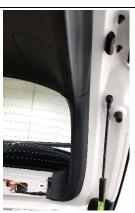
3. Some models may have a clip that holds the rear panel on, remove that at this time and gently pull straight off the hatch, it helps to start at one corner and work your way over to the other side
