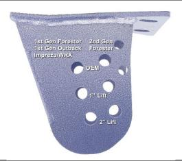
5. Install the supplied bolt, spacer and nut for the emergency brake cable in the appropriate hole.
