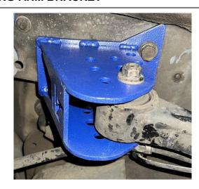
4. Reinstall trailing arm into the appropriate hole in the bracket, see picture for trailing arm location
