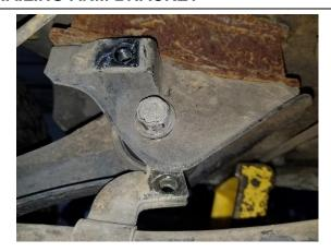
2. Remove the 3 bolts that hold the trailing arm bracket to the chassis. Retain the bolts for step 3.
