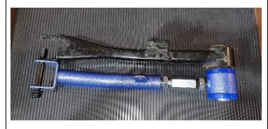
7. Install the trailing arm on the subframe side first, once the trailing arm is on the pin, install the included M14 fender washer and the factory bolt.
