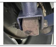
9. Set the car on the ground, settle the rear suspension and torque the bolts to the following torque specifications:
