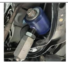
8. Install the trailing arm to the knuckle using the factory bolt
