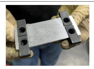
9. Pass the oil filter drain panel mounts through the skid plate as shown and secure to the plate with supplied button head fasteners
