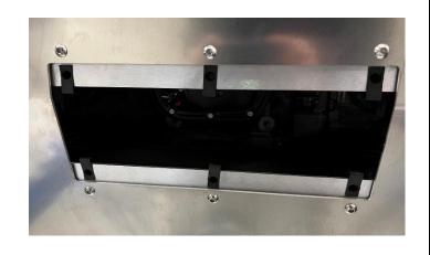
8. Place the u-nuts on the oil drain panel mounts as shown
