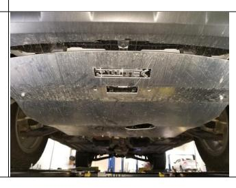
4. Move to the rear of the skid plate and install the 50mm long bolts and nuts to the tabs on the transmission cross member. NOTE: Tighten the front bolts first and the rear bolts second.
