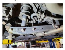
Compress spring, making sure all spring pressure is removed from upper spring seat and an air gap exists. Follow all spring compressor manufacturer instructions and safety measures.
