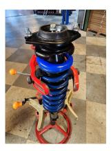
Remove upper strut nut and replace old spring with new RalliTEK spring, making sure the logo and part number are right side up. If the rear springs require strut extensions they will be included. Please reference RTEK-100074 for strut extension installation.
