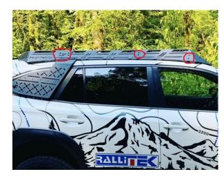
Now, using the bag labeled "siderails" you can attach the side rail to front, middle, and rear brackets, using 1 washer, 1 lock washer and 1 screw per hole as shown in photo. Leave these screws snug but not fully tightened to allow movement.
