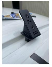
Next, you will Install the rear, middle and front roof brackets on top of the nylon spacers in the corresponding spot (rear bracket for the holes closest to the back of the vehicle, mid one in the center of vehicle, and front bracket in front of vehicle) using 1 small washer and 1 m6 screw per hole.
