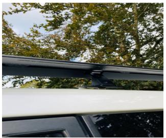
Next, take the corresponding side-rail and slide it into the rear, middle and front brackets that you have installed on the roof. The brackets will slide into the side-rail slots.
