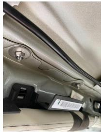
Now, you will remove 4 nuts and 4 large washers from the hardware bag labeled "roof brackets". Then you will be applying the nut and washer to the inside of the interior/underside of the roof to secure the screws, as shown in the photo. At this time leave these snug but not fully tightened. (allowing movement for slight adjustment...you will tighten later).
