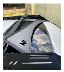
After both side rails have been installed, locate the wind fairing and hardware bag labeled "wind fairing". Slide wind fairing in behind both front corners of the side rails as shown in the photo. Line up the holes of the wind fairing and side rails and attach them using 1 screw, 1 washer and 1 lock washer per hole. Leave screws loose for now. You will tighten these after crossbars are installed.
