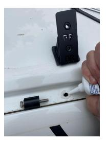
Next, you will be adding waterproof caulking around each hole. Then you will place one nylon spacer firmly down and centered over each hole as shown in the photo below. You will do this for every hole (where a bracket is to be installed) This is important to keep water out of your cabin. Don't be worried about using a little extra caulking where you think it may need to be added.
