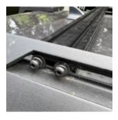
Now, locate all 6 crossbars and hardware bag labeled "crossbars". Then, drop all 6 crossbars in between side-rails, aligning them with side-rail slots, as shown in the photo. Add hardware (1 washer, lock washer and screw per hole) and fully tighten.
