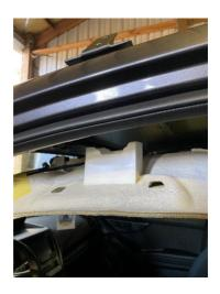
Before getting started with install, you'll need to remove (drop) your interior headliner and remove the stock roof rack. The process is actually fairly simple. We recommend watching a few "how -to" videos on youtube. Just search "Crosstrek remove stock roof rails" or "Crosstrek headliner drop" and watch a few of the videos to learn how to do this part. There are several that demonstrate how to do this.
