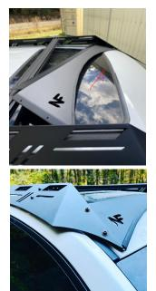
After both side rails have been installed, locate the wind fairing and hardware bag labeled "wind fairing". Slide wind fairing in behind both front corners of the side rails as shown in photo. Line up the holes of the wind fairing and side rails and attach using 1 screw, 1 washer and 1 lock washer per hole. Leave screws loose for now. You will tighten after crossbars are installed.
