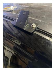
Next, you will Install the rear, middle and front roof brackets on top of the nylon spacers in the corresponding spot (rear bracket for the holes closest to the back of the vehicle, mid one in center of vehicle, and front bracket in front of vehicle) using 1 small washer and 1 m6 screw per hole.
