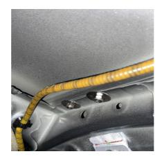
Now, you will remove 6 nuts and 6 washers from the hardware bag. Then you will be applying the nut and washer to the inside of the interior/underside of the roof to secure the screws, as shown in the photo. At this time leave these snug but not fully tightened. (allowing movement for slight adjustment...you will tighten later).
