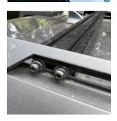
Now, locate all 7 crossbars and hardware bag labeled "crossbars". Then, drop all 7 crossbars in between side-rails, aligning them with side-rail slots, as shown in the photo. Add hardware (1 washer, lock washer and screw per hole) and tighten. \*\* IF YOU HAVE THE LIGHT BAR WIND-FAIRING OPTION BE SURE TO COMPLETE THE FIRST STEP BELOW PRIOR TO INSTALLING THE CROSSBARS, AS THE FRONT CROSSBAR WILL NEED T-SLOTS ADDED FIRST IN ORDER TO
