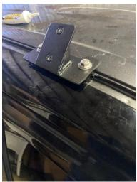
Next, you will Install the rear, middle and front roof brackets on top of the nylon spacers in the corresponding spot (rear bracket for the holes closest to the back of the vehicle, mid one in center of vehicle, and front bracket in front of vehicle) using 1 small washer and 1 m6 screw per hole.
