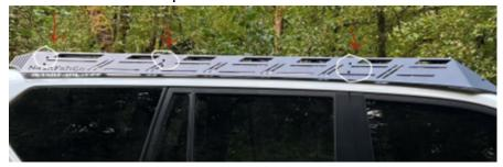
Once you have installed one side rail for one side of your vehicle, you will **go back to the first** steps and <u>repeat this process for the other side of your vehicle.</u>
