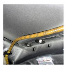
Now, you will remove 6 nuts and 6 large washers from the hardware bag. Then you will be applying the nut and washer to the inside of the interior/underside of the roof to secure the screws, as shown in the photo. At this time leave these snug but not fully tightened. (allowing movement for slight adjustment...you will tighten later).
