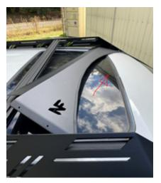
After both side rails have been installed, locate the wind fairing and hardware bag labeled "wind fairing". Slide wind fairing in behind both front corners of the side rails as shown in photo. Line up the holes of the wind fairing and side rails and attach using 1 screw, 1 washer and 1 lock washer per hole. Leave screws loose for now. You will tighten after crossbars are installed.
