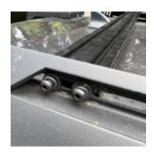
Now, locate all 5 crossbars and hardware bag labeled "crossbars". Then, drop all 5 crossbars in between side-rails, aligning them with side-rail slots, as shown in the photo. Add hardware (1 washer, lock washer and screw per hole) and tighten.
