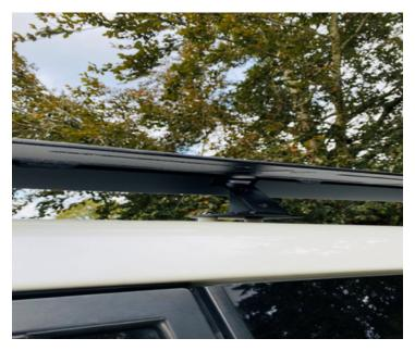
Next, take the corresponding side-rail and slide it into the rear, middle and front brackets that you previously installed on the roof. The brackets will slide into the side-rail slots.
