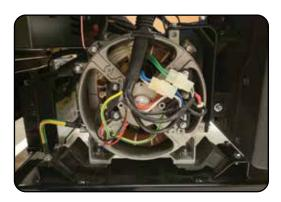
The carbon brushes in conjunction with the AVR regulates power from the generator. The carbon brushes are wearable parts and should be inspected every 250 running hours.
