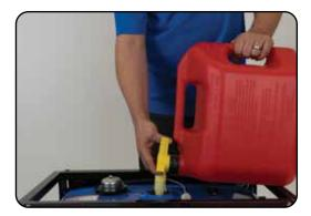
If you have been using gasoline in your generator, before storing your generator for extended periods of time you should drain your generator fuel tank of gasoline.
