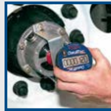
Install DataTrac Pro on wheel end.
