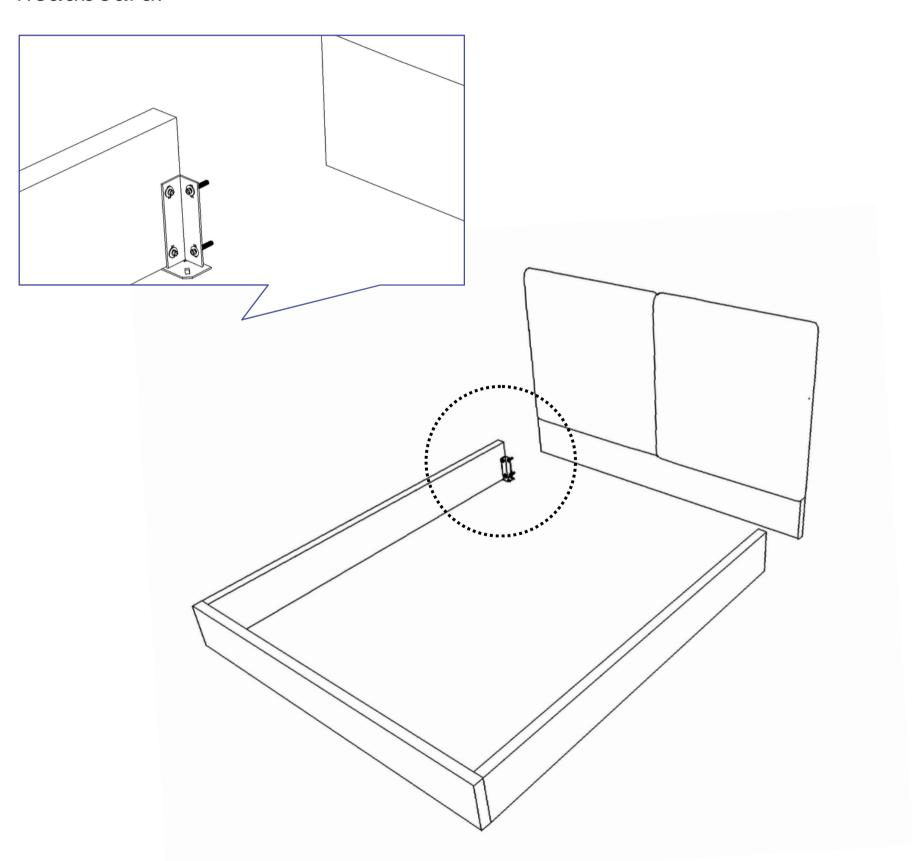
Use M8-50 Truss Head screws to fix the bedside support with right and left side of bottom shroud.
