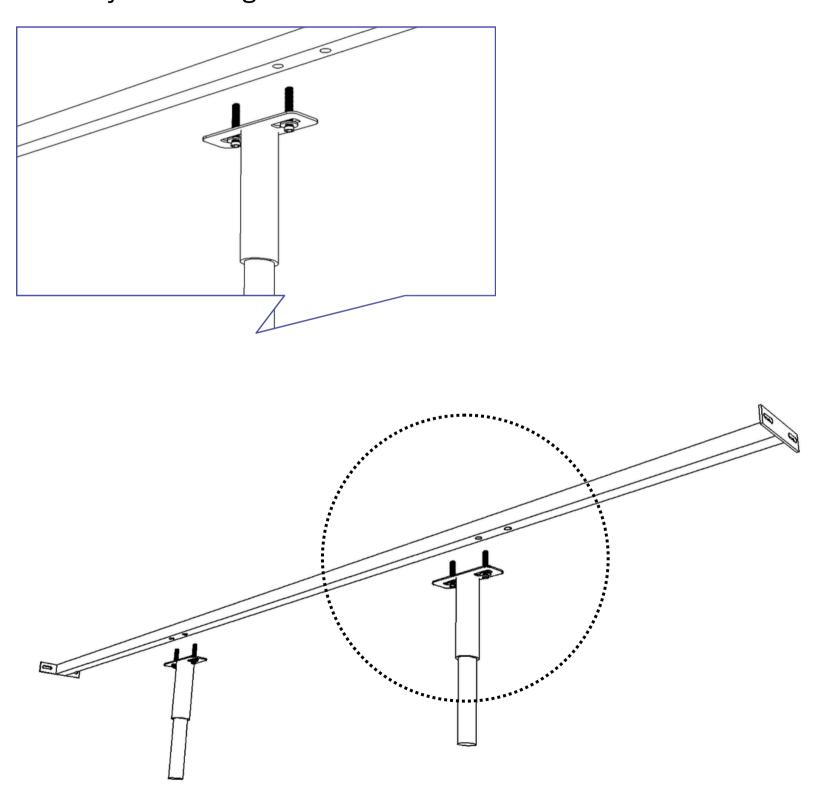
Use M8-40 Truss Head screws fix both bedside support with headboard and bottom shroud.
