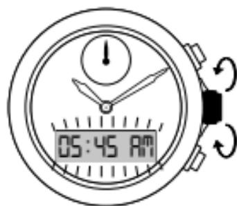
Turn crown C **slowly** in either direction to activate the EL backlight of the LCD.
