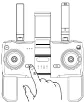
Press the Return Home button on your transmitter or select this feature from your smartphone. The transmitter will begin beeping. The aircraft will return to the original point of take-off. Press the button again to halt the RTH procedure or alter the left and right joysticks to force the aircraft to land elsewhere.
