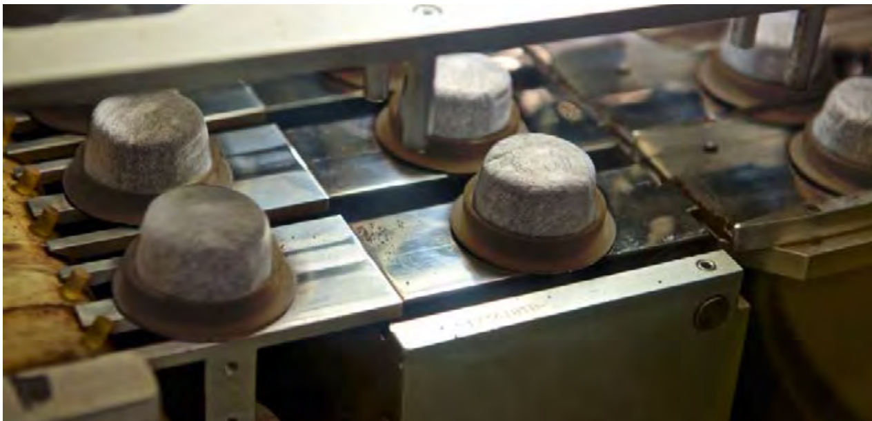
A close-up view of the compostable PurPod100 coffee capsules running through their packaging steps at the Club Coffee plant.
