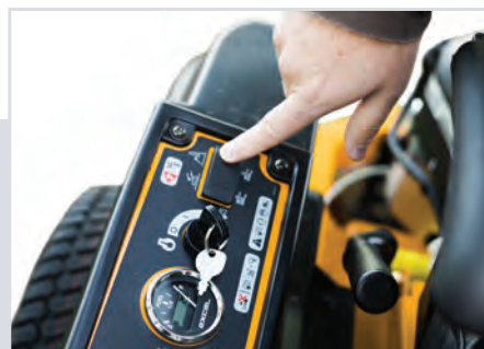
Auto Deck Height Adjustment Raises and lowers deck with the push of a button.
