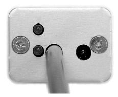
Fig. 36 - indicators, cable and power supply connector
