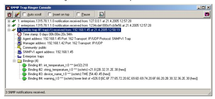
Fig. 33 – Trap 1 – the temperature value occurs below the lower limit
