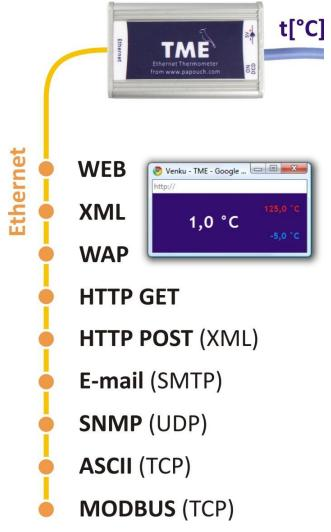
Fig. 3 – Temperature acquisition method
