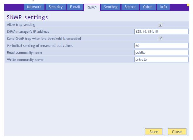
Fig. 14 - SNMP settings panel
