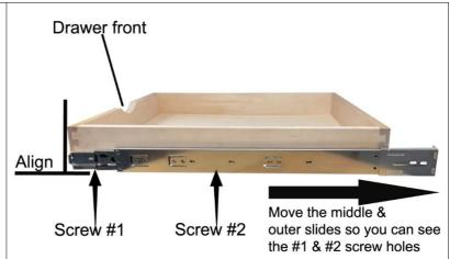
Note: Make sure the both sides of the slides are secured horizontally parallel on the drawer
