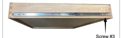
Note: Make sure the both sides of the slides are secured horizontally parallel on the drawer
