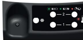
4. When the LEDs turn off, the charger is ready for use.
