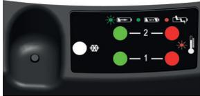
3. When powered on, the charger initialises: Green LED + Red LED light for 2 seconds.
