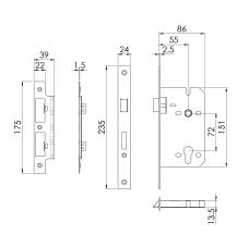
Contract Din Euro Profile Sashlock, 55mm. Square or Radius option. The Latch bolt has the Easi-T reverse function to save undoing the case so it can be reversed in seconds. Certified to BS EN 12209.
