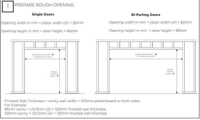
**Note:** When installing a bi-parting kit, please repeat the installation on the opposite side, unless otherwise stated.
