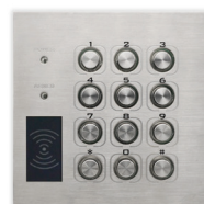
MEM-KP02 Digital Keypad Module 26-bit Wiegand Output
