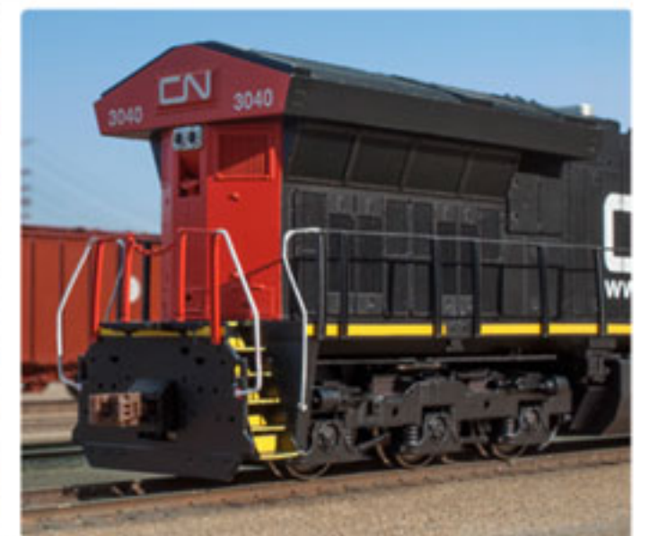
Spotting Feature: Large Triangular Radiator
