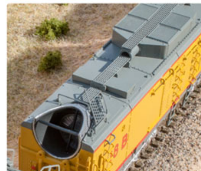
H-H, H-I, I-I dynamic brake configurations
