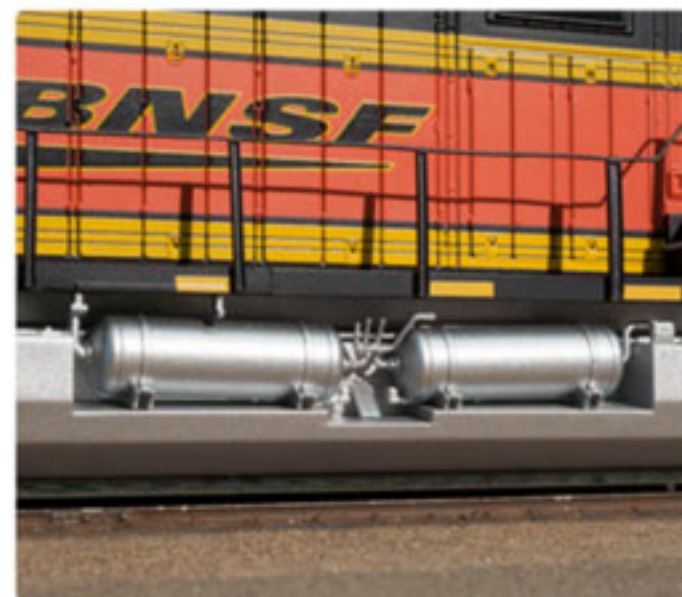
Separate Air Tanks
