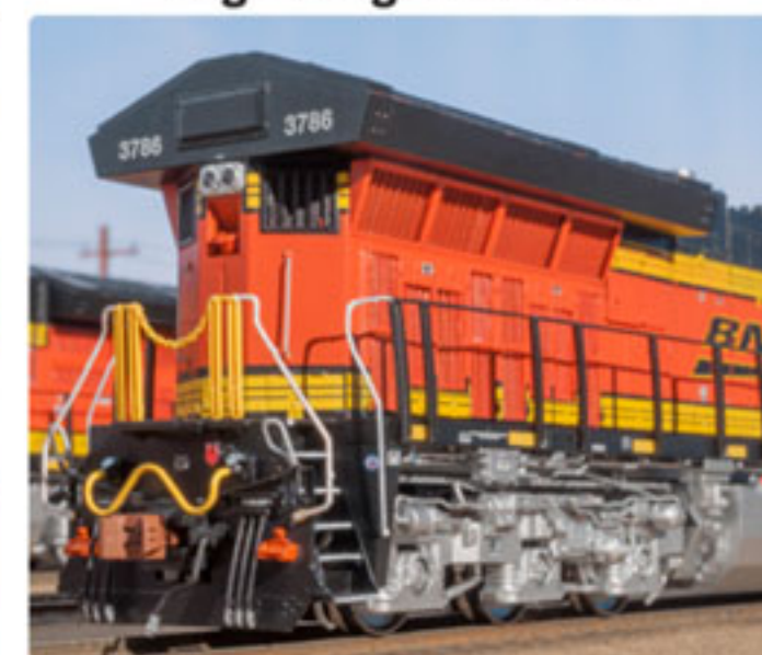
Spotting Feature: Large Triangular Radiator
