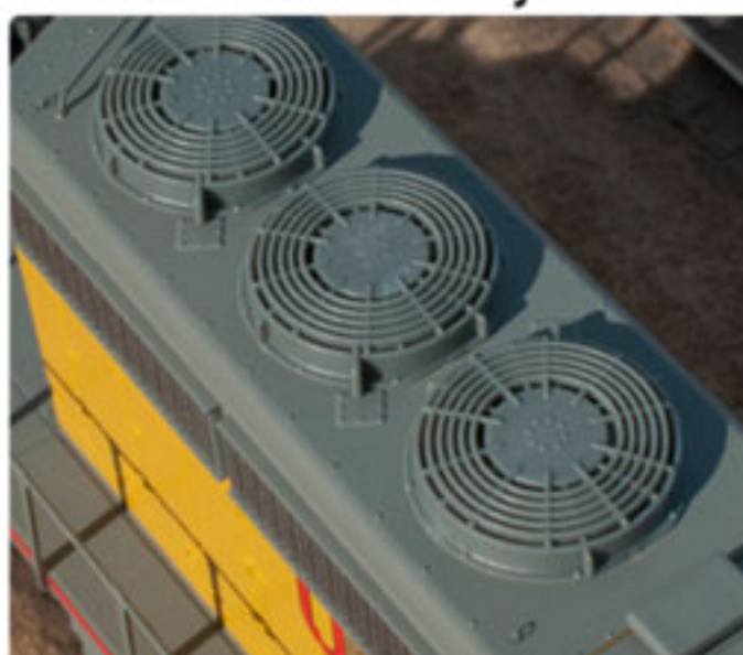
48" radiator "Q" fans
