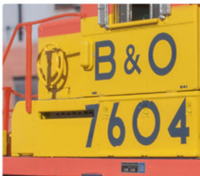
Chessie mailslot battery box doors
