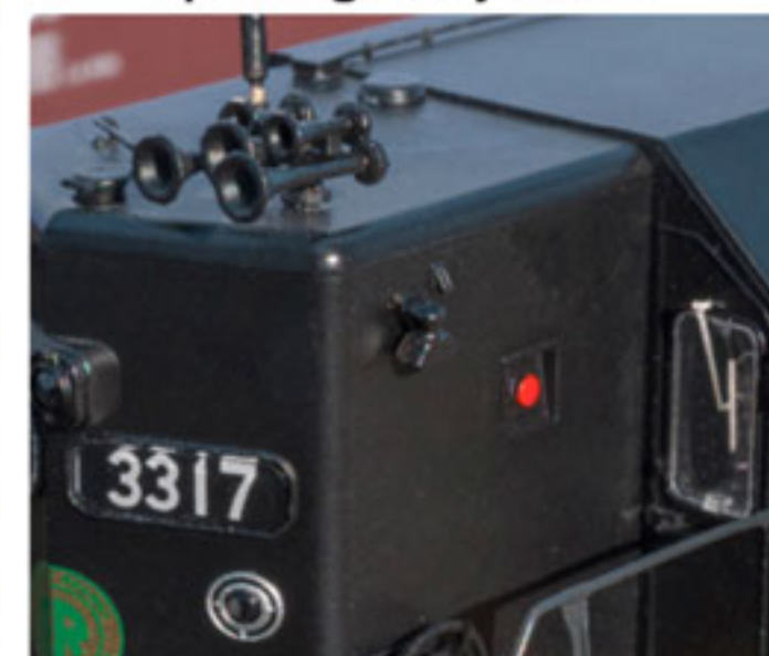
Southern walkway lights
