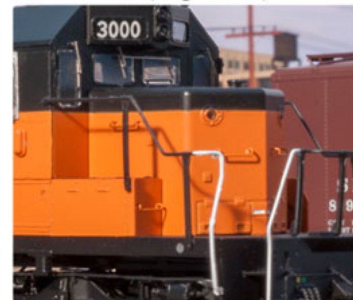
Operating flush mount tri-color class lights
