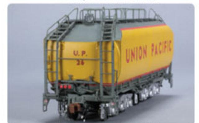
Detailed rear end of the 23C tender, showing its operating back-up light, and separately applied plumbing details.
