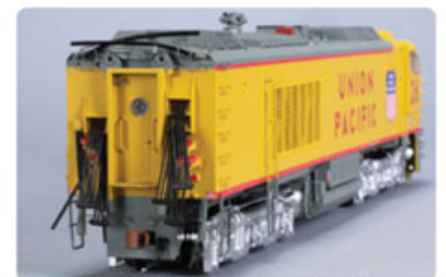
Rear of GTEL A-Unit 26B showing the flexible rubber electrical bus cables and MU cables for installation between the A and B-unit
