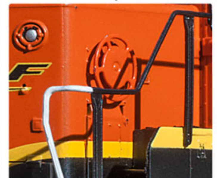
88" nose with brakewheel
