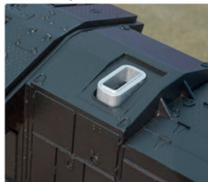
Angled Engine Exhaust Cab
