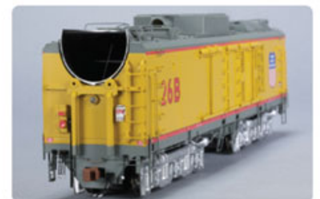
Rear of GTEL B-Unit #26B, showing the rear of the rooftop "Dynavane" air intake system, operating back-up light, and exhaust housing.
