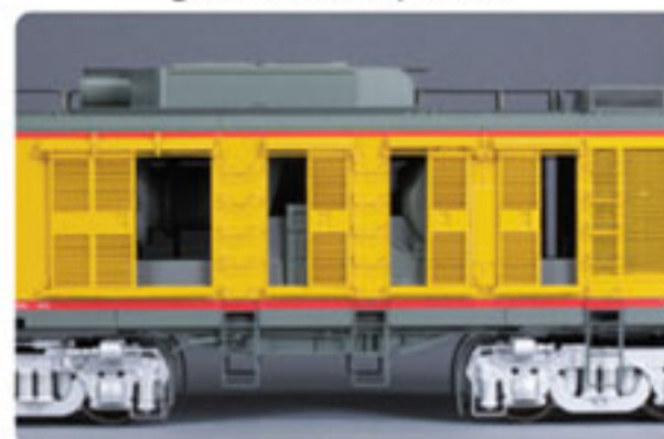
Open B-Unit doors revealing a replica of a GE 10-chamber centrifugal-flow gas turbine and accompanying generators.
