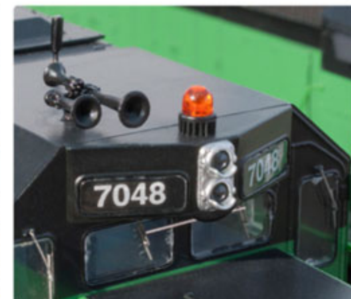
Operating rotary beacon
