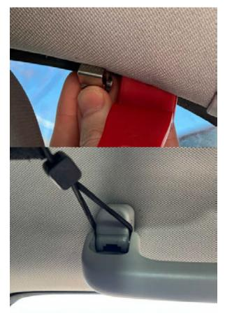
6. Take your panel removal tool and slide it into the sides of the back of the headliner, creating space for you to slide the black clips onto the headliner. Clips should be located on the far ends of each side of the headliner, and an inch from either side of the rear window. For the middle two clips you may need to insert the panel tool farther out on the sides and slide it over to the window. Slide the larger end of the clip onto the headliner.
