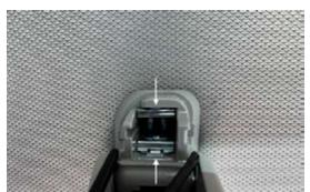
1. Remove plastic cap covering rear hinge of rear passenger handles using a pick or screwdriver to gain access to the metal clips attaching them to the ceiling. Pull out and towards you on the side where the notch is located. Be careful as you use your tool to not damage the plastic.
