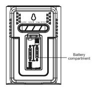
Step 1, Remove the battery compartment cover and insert 2xAAA batteries.
