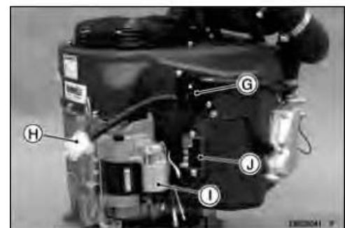
G. Fuel Pump H. Fuel Filter I. Electric Starter J. Voltage Regulator
