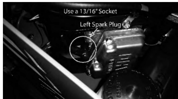
Spark Plug Component and Details
