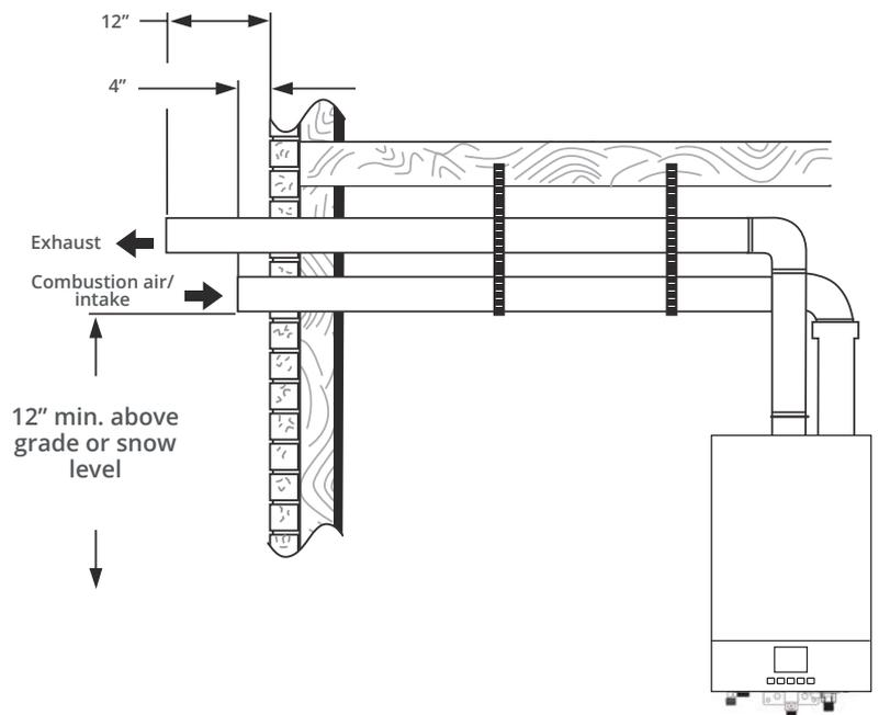
The vent termination and air intake must be in the same pressure zone and face the same direction.
