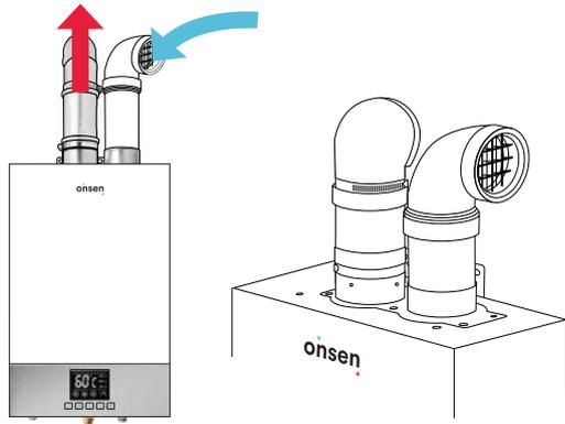
**Figure 2: Example of Air Intake Pipe Configuration**
