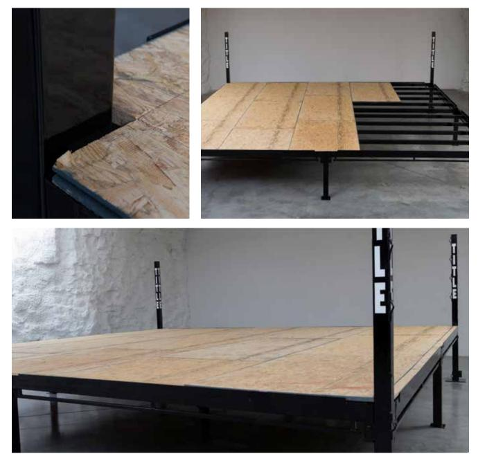
Tighten turnbuckles in all 4 corners until ring posts lean out a bit. Measure with square ruler. Ring post should lean out about ¾<sup>~</sup>at the top of the square ruler.
