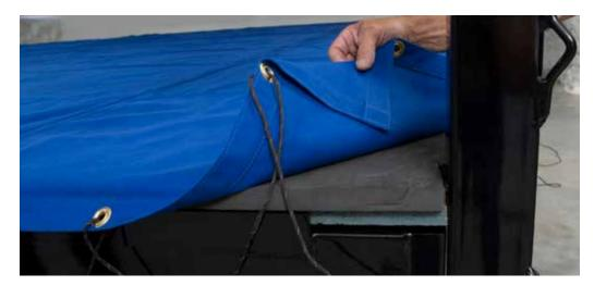
After running the rope thru Side 1, do the side directly opposite (Side 2 in diagram). This will make sure the canvas is pulled tight. Then complete the remaining two sides. Once all four sides have rope and are tight, cut the rope at the corners and tie tight on bottom bar.
