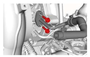
**Step 20**: Unbolt coolant return line from the turbo charger.
