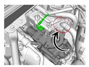
**Step 9**: Disconnect EGR connector and remove the coolant pipe that is attached to the cooler.
