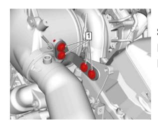
**Step 25**: Remove the downpipe bracket bolts and discard the bracket.
