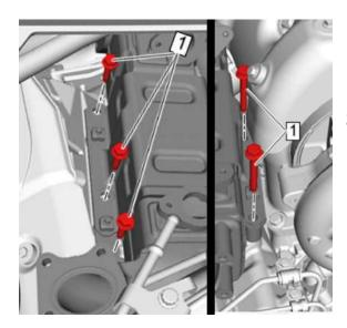
**Step 12**: Unbolt EGR Cooler and remove assembly.
