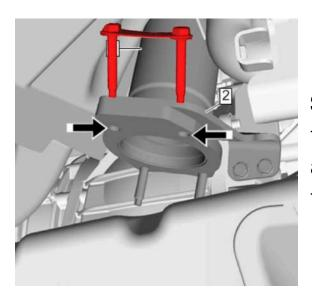
**Step 26**: Remove 4 downpipe to front pipe mounting nuts & studs and remove factory downpipe from the vehicle.
