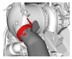
**Step 23**: Undo v-band clamp that attaches the turbo to the catalytic converter. Undo 4 hold down bolts for the turbo and remove the turbo.
