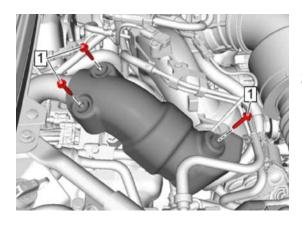
**Step 6**: Remove EGR Valve pipe heat shield
