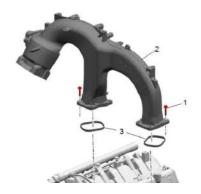
**Step 8**: Unplug all electrical connectors, unclip wiring harness, unbolt coolant line support bracket and disconnect the line to move it out of the way. Remove the 8 bolts that hold the upper
