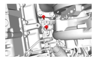
Step 22: Unbolt oil drain pipe.
