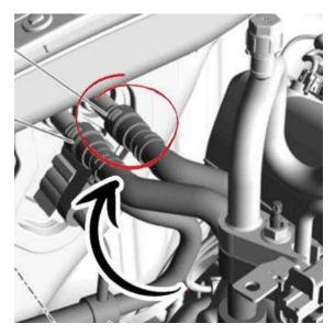
**Step 15**: Remove the circled heater core hose that is closest to the engine. Remove the hose from the fitting and reuse factory fitting, attach it to the provided coolant hose.
