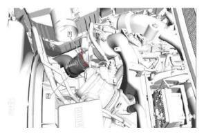
**Step 5**: Disconnect charge air cooler outlet to upper intake manifold.
