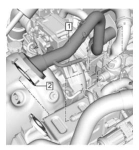
**Step 10**: Remove EGR Cooler coolant feed pipe. Remove rubber hose off the end for reuse.
