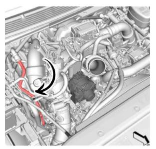
**Step 18**: Unbolt and remove coolant hose assembly
