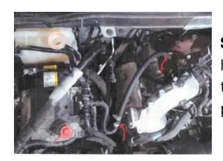
**Step 31**: Replace factory coolant hose with provided coolant hose that has a preinstalled barb as pictured.
