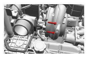
**Step 18**: Unbolt PCV hose from the turbocharger and reposition it out of the way.
