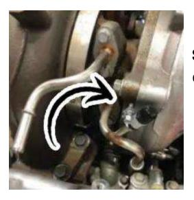
**Step 29**: Install supplied rubber coolant cap.
