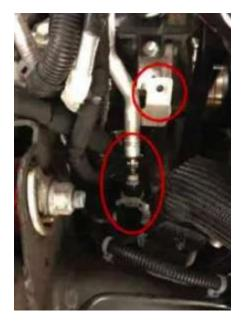
**Step 19**: Install the larger supplied hose that has a preinstalled barb. On the upper side use the provided quick connect fitting, connect the bottom side to the fitting shown in the photo, with supplied hose clamp.
