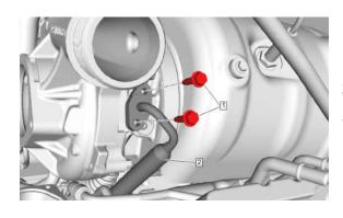
**Step 19**: Unbolt oil feed pipe from turbocharger
