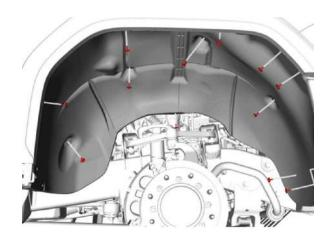
**Step 17**: Remove passenger side fender liner.
