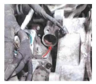
**Step 14**: Install provided coolant block off plug with 0-ring in this location.
