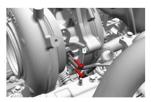
**Step 21**: Unbolt coolant feed line from the turbo charger.
