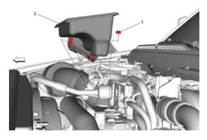
**Step 2**: Remove air cleaner outlet resonator.
