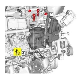
**Step 13**: Remove EGR Valve, install supplied block off plate and gasket.
