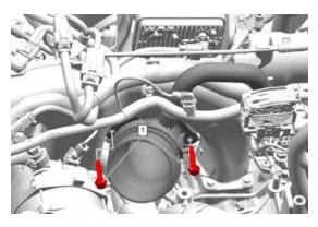
**Step 4**: Remove turbocharger air inlet adapter and move it out of the way carefully as these are not serviceable.
